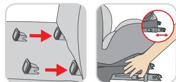
The ISOFIX mounting points are located between the seat and the backrest of the car seat.
