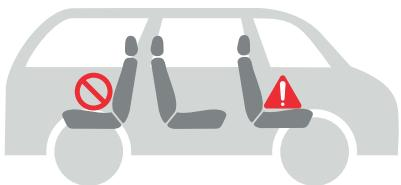
For securing the child car seat with ISOFIX and Top Tether there is a "universal" approval. For this reason, these seats can only be used in certain cars. Please check the approved vehicles based on the vehicle type list. A current list can be found at [www.h-germany.de](http://www.h-germany.de)
