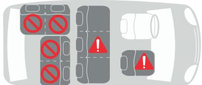
Use the vehicle type list of your manufacturer to check which vehicle seats are suitable for child car seats.
